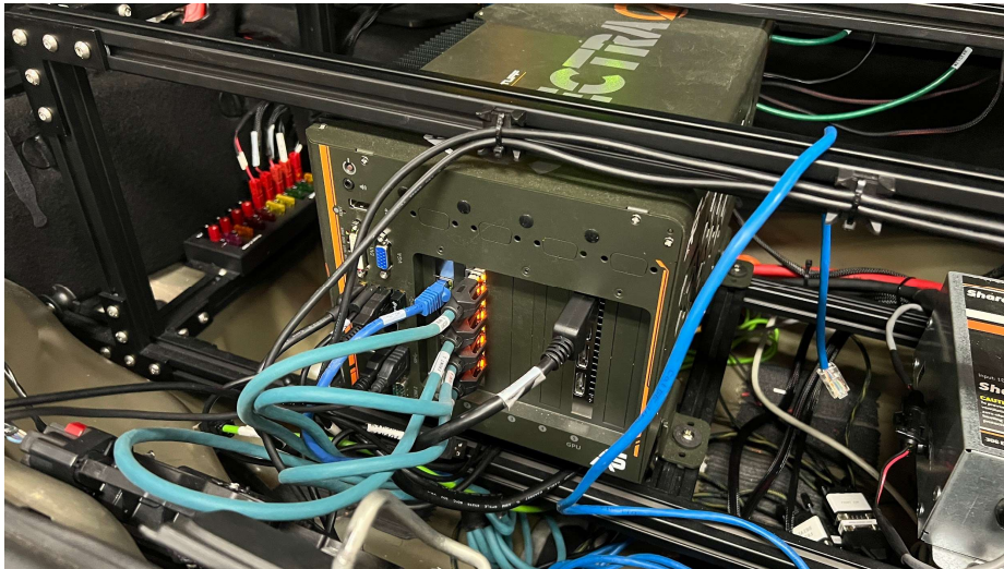
Figure 7: Rear I/O of the PC with USB, Ethernet, and graphics ports
